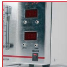
With its own LED displays and calibration controls, the FerMac 368 can be used with any size or make of bioreactor. It does not require complex installation and can be used either as an independent instrument or through existing fermentation software.
